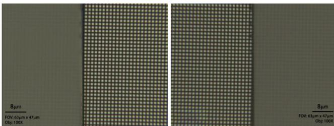
**Figure 3.** ZDot technology maximizes signal strength at multiple focal planes in order to provide accurate step height measurements. The left image shows the ZDot grid in focus at the top surface of the step (right side of image), and the right image shows the grid in focus at the bottom surface of the step (left side of image).
