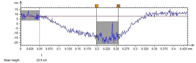
Figure 8. Shallow SIMS crater with 23nm depth measurement.
