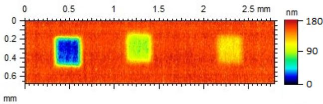
Figure 5. Top-down 3D image of multiple SIMS craters with varying depths.
